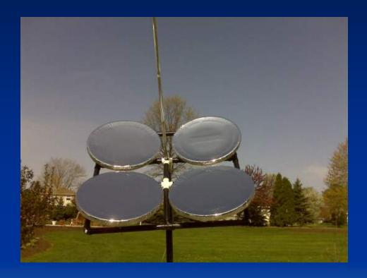
• And constructed a ¼ scale model of a 4-dish tracking structure
